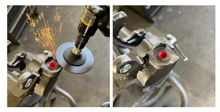
**For high-offset 6-lug kits optioned with standard rubber hoses**, the hoses are a tight fit. To help with fitment, you can sand the boss on the caliper in order to clock the banjo fitting on the caliper slightly to clear the spacer. Pay close attention to sand the boss **only** and **not** the sealing surface for the crush washer.
