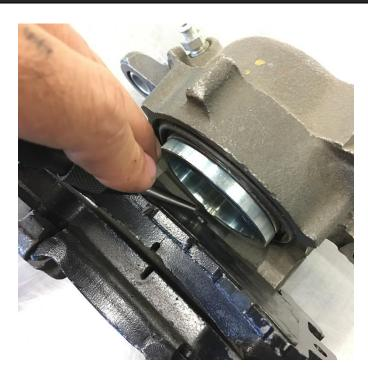
**5-lug kits with non-parking brake calipers** should be checked to confirm the machined pad spacers are present **(6-lug kits do not use these)**. Make sure the notch lines up with the corresponding boss on the brake pad.
