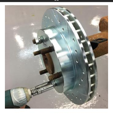
The rotor can now be installed using 2 lug nuts to temporarily secure it. In the case of drilled/slotted rotors, the direction of rotation shown is for the **passenger side**. **NOTE:** Verify that the rotors are sitting flat against the axle shaft.
