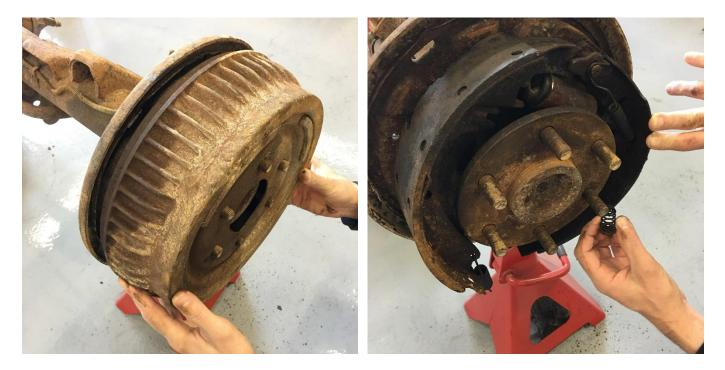
This installation refers to both 5-lug and 6-lug axles, and to the **passenger side** of the axle. All steps are to be repeated on the driver side. Start by removing the factory drum. It may be necessary use a lubricant around the axle register to do this. Once the drum is removed, remove the brake shoe retaining springs (2 places) as shown.
