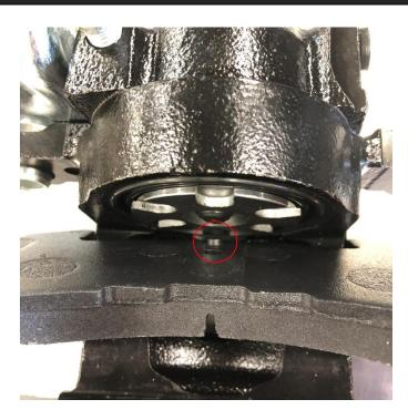
**5-lug and 6-lug kits with parking brake calipers** should be checked to confirm the pad is seated flat against the piston face, with the boss of the brake pad lining up with the notch in the piston face.
